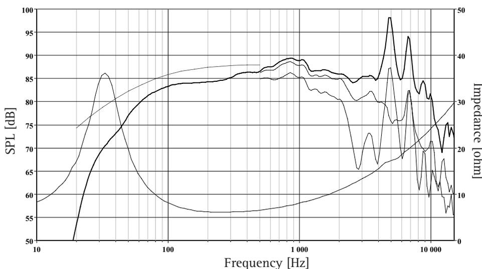
The frequency responses above show measured free field sound pressure in 0, 30, and 60 degrees angle using a 20L closed box. Input 2.83 V<sub>RMS</sub>, microphone distance 0.5m, normalized to SPL 1m. The dotted line is a calculated response in infinite baffle based on the parameters given for this specific driver. The impedance is measured in free air without baffle using a 2V sine signal.
